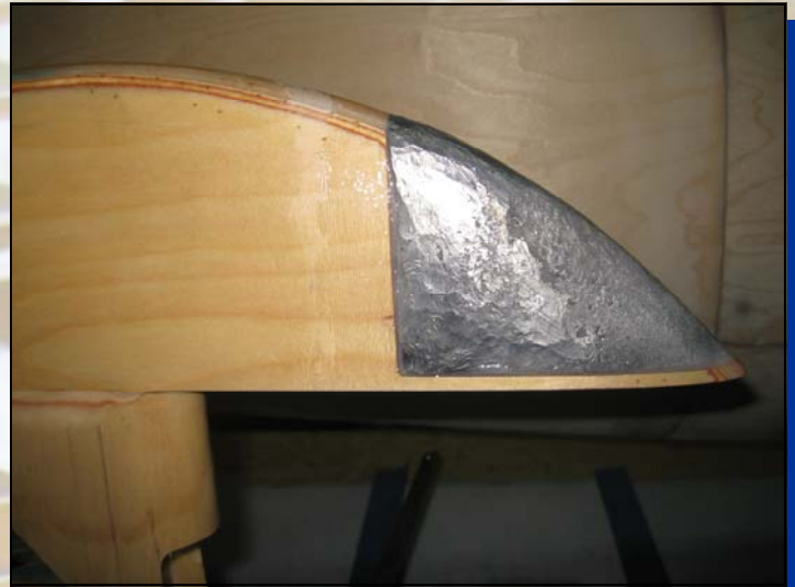
Counter weight glued and screwed in place. This will all be covered with filler.
