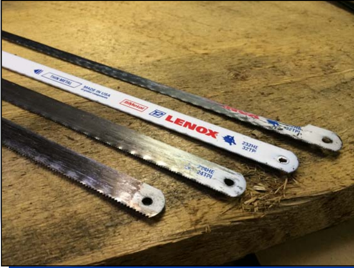
Comparison of different blade pitches; left to right, 18, 24, 32, 32. Blade on far right has been ground to allow curved cuts
