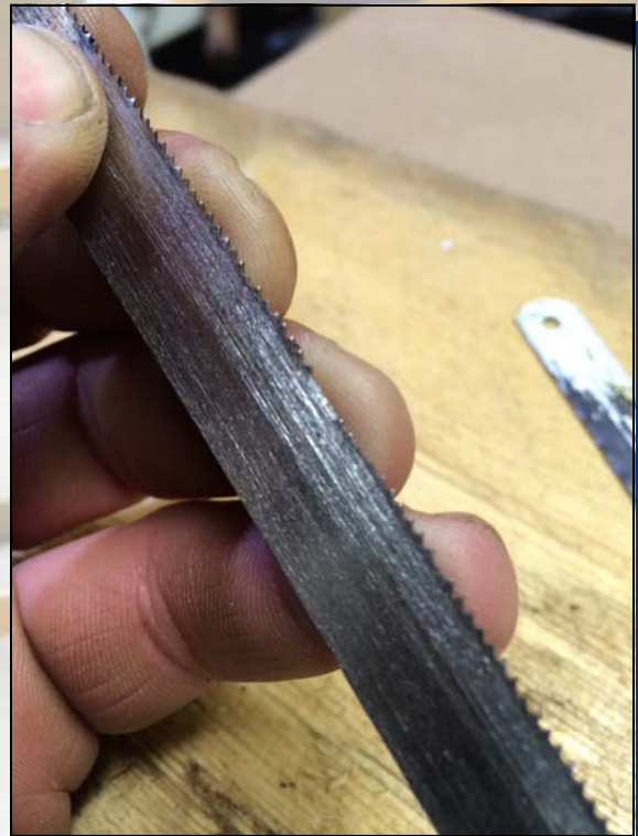
Section of broken teeth from cutting too thin material
