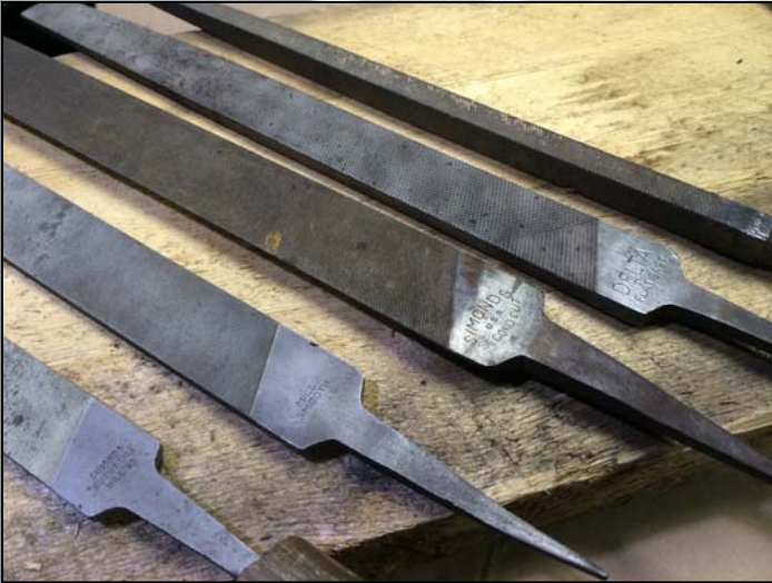
Shapes and cuts of files: 2 mill, half round, flat, square
