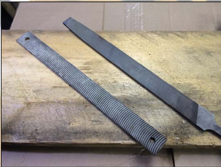
Vixen file with curved teeth for aggressively removing soft material, pictured next to 12" mill bastard.
