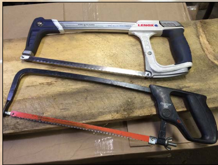
Compared to a cheap frame that gives hacksaws a bad name. Blades are both 12"
