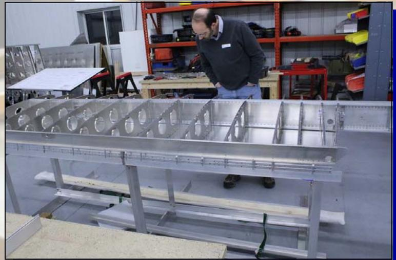
Me looking at the riveted sandwich spar buildup on one of the fastbuild kits. They keep the 51% rule—just barely!
